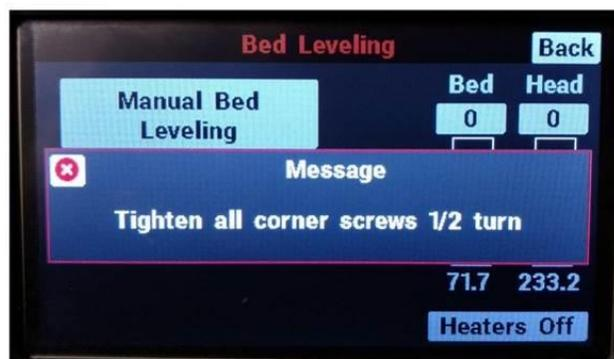
**Note:** If your bed is very out of level and you are running through this wizard multiple times in a row, DO NOT tighten all the corner clips on your 2<sup>nd</sup>, 3<sup>rd</sup>, etc runs.
